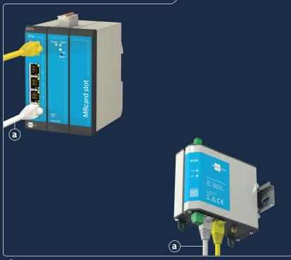
(a) Connect router to the network that is used to establish the **Internet connection** (MRX/MRO: ETH 5, ECR/SCR: ETH 2)
