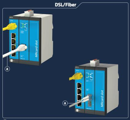
(a) Connect DSL connection line / SFP module with glass fiber line to the VDSL/ADSL or SFP 1 socket
